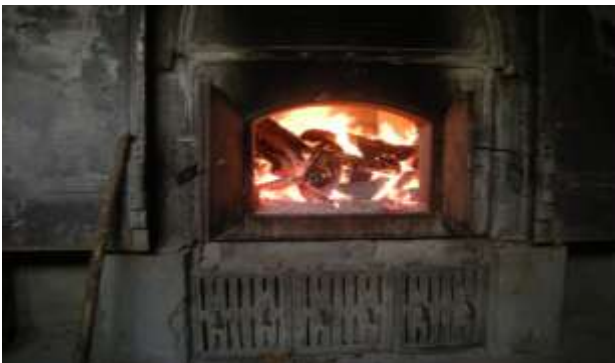
Plate 5 Flame get sucked in towards left hand side
