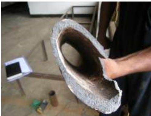
Plate 7 Uneven thickness of an oval tube
